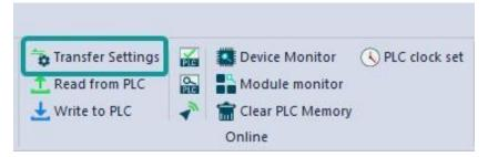
3 The "Transfer settings" dialog box pops up, when the "Detailed settings" is not checked, select the specified port, it is as shown in the figure below.
